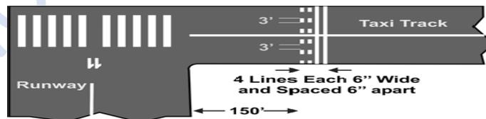
(b) **Runway Holding Position Markings.** These markings shall consist of four lines of 0.15 m (6") width each with spacing of 0.15 m (6").
