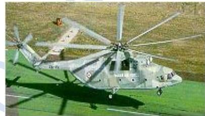
22. **MI-26** : Twin engine turboshaft, military heavy lift helicopter of Russian origin with carrying capacity of 70 combat equipped troops or 20,000 kg payload.
