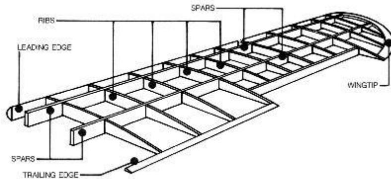
8. As shown in figure above, a wing is a type of fin with a surface that produces lift for flight or propulsion through the atmosphere, or through another gaseous or liquid fluid. As such, wings have an airfoil shape, a streamlined cross-sectional shape producing a useful lift to drag ratio.
