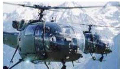
25. **CHEETAH** : Single engine turboshaft, helicopter of French origin having capacity to carry 3 passengers or 1000 kg external sling loads. Cheetah is the life line of the Siachen Glacier dropping load and evacuating soldiers from the highest battlefield in the world.
