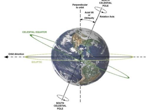
16. **Latitude.** These are the angular distances along the meridians. The latitude of a place is defined as the arc of its meridian between the equator and the place and is named North or south depending upon its corresponding position in respect to the equator. The latitude is measured in degrees, minutes and seconds from  $0^\circ$  to  $90^\circ$  from the equator.
