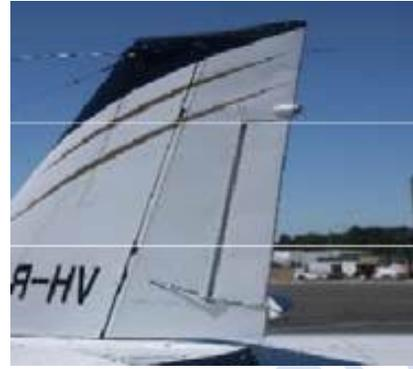
15. The rudder is a fundamental control surface, typically controlled by pedals rather than at the stick. It is the primary means of controlling yaw—the rotation of an airplane about its vertical axis. The rudder may also be called upon to counter-act the adverse yaw produced by the roll-control surfaces.
