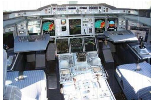
15. A glass cockpit is an aircraft cockpit that features electronics instrument displays rather than mechanical gauge .It is as simple as that. A glass cockpit uses displays driven by flight management system that can be adjusted to displays flight information as needed. This simplifies aircraft operation and navigation and allows pilot to focus only on the most pertinent information. They are also popular with airlines companies as they usually eliminate the need for a flight engineer.
