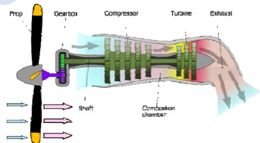
19. The main difference between single shaft and free turbine engine is in the transmission of power to the propeller.
