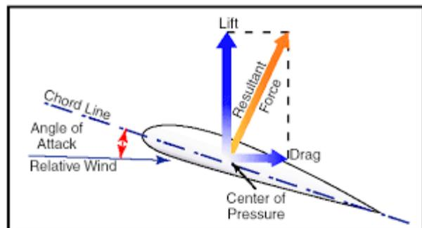
26. **Angle of Attack.** It is the angle between the chord line and the relative air flow undisturbed by the presence of aerofoil.
