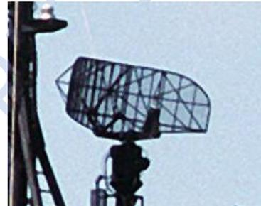
4. Radar is an object detection system which uses radio waves to determine the range, altitude, direction, or speed of objects. It can be used to detect aircraft, ships, spacecraft, guided missiles, motor vehicles, weather formations, and terrain. The radar dish or antenna transmits pulses of radio waves which bounce off any object in their path. The object returns a tiny part of the wave's energy to a dish or antenna which is usually located at the same site as the transmitter.
