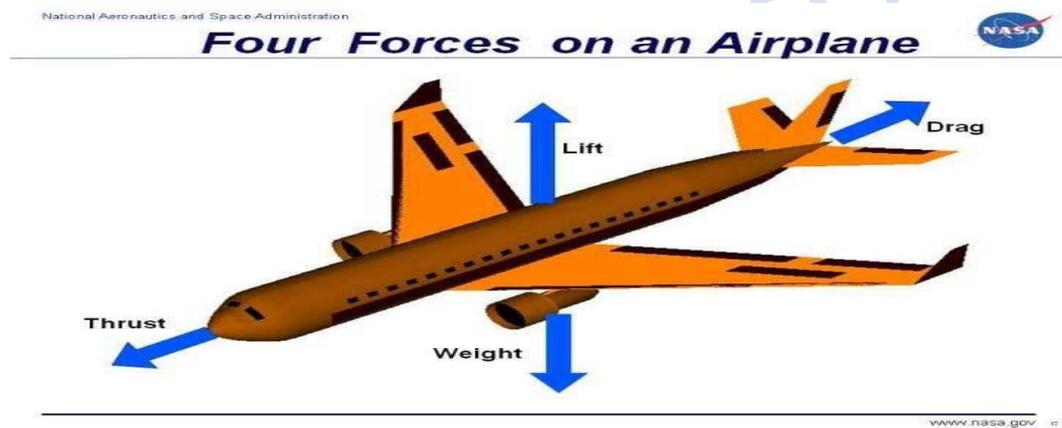
***Lift and Drag are the most important components of aircraft in level flight. They act in  $90^{\circ}$  to each other. The Lift component of aircraft supports the aircraft in air whereas the drag resist the aircraft movement in air.***
