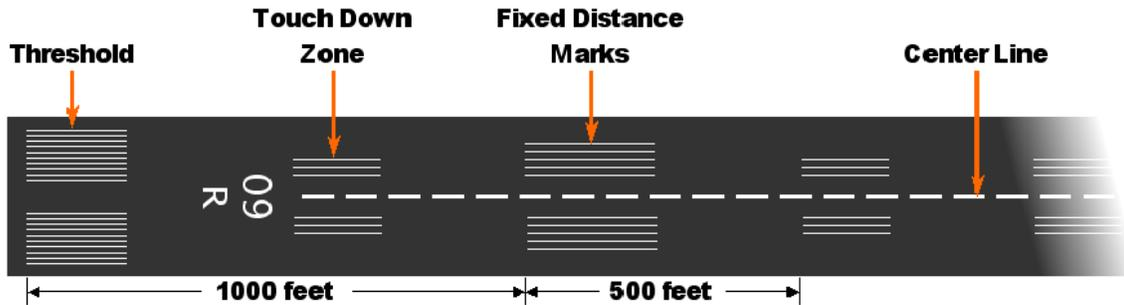
(b) **Runway Centre Line Markings.** Runway centre line markings shall consist of a series of broken longitudinal lines along the runway centre line and extending along the whole length of the runway
